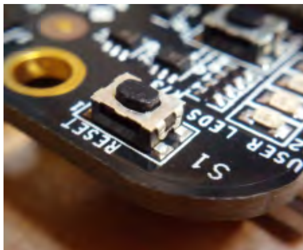
Figure 3. The reset switch is in the corner of the board at the Ethernet adapter end.
