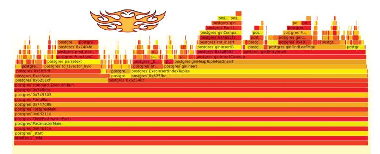
Example of a flame graph generated from PostgreSQL, generated using output from DTrace one liner:
