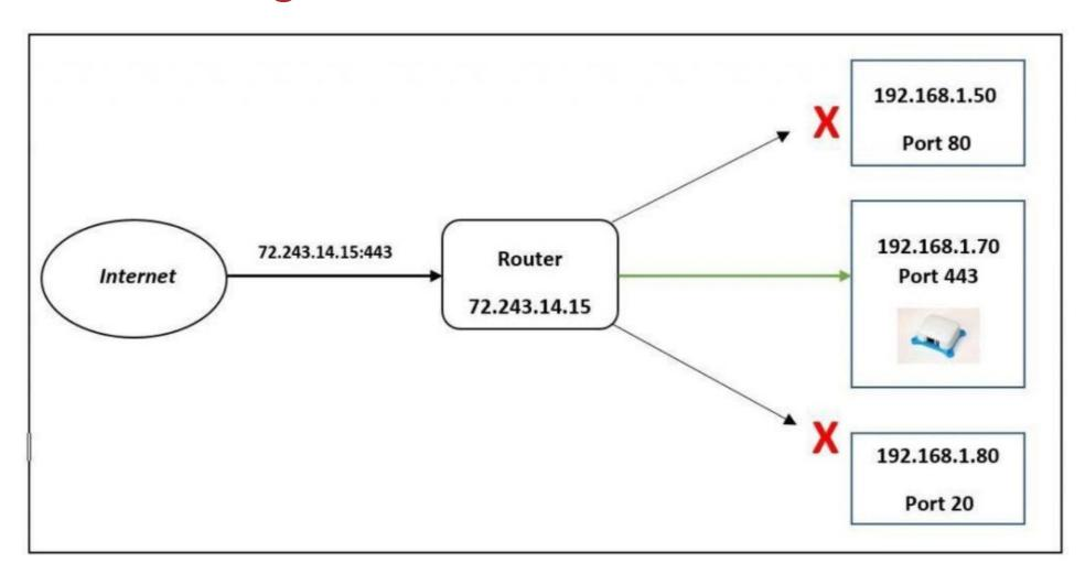
The next step is to make sure that the router connected to the device is properly forwarding all Minecraft traffic to the device. Even if there are no other computers on the network, this is a
