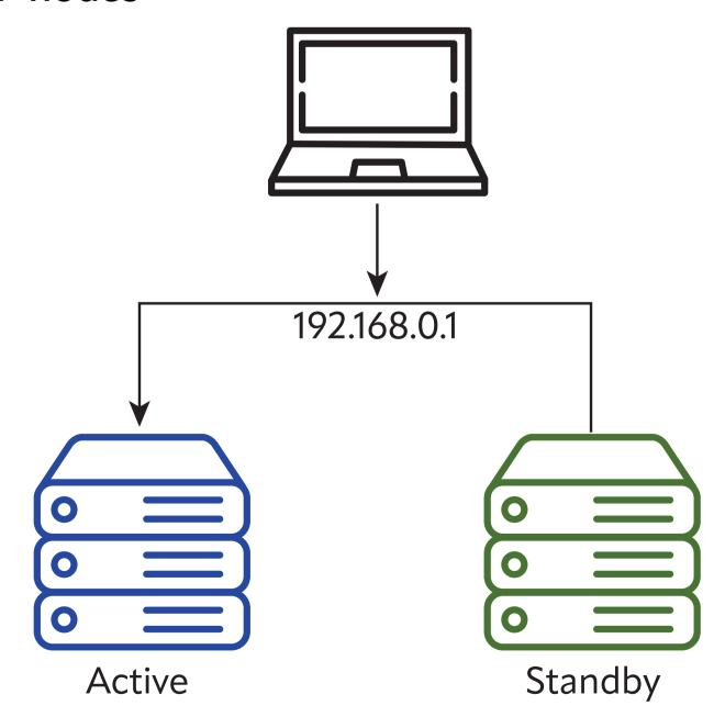
In CARP, the active node is broadcasting its activity. This process is shown in Figure 2. Because the blue host is an active node, it is broadcasting CARP packages. The green and orange nodes are on standby and do not send any packages. The CARP package is quite small and contains only minimal information like:
