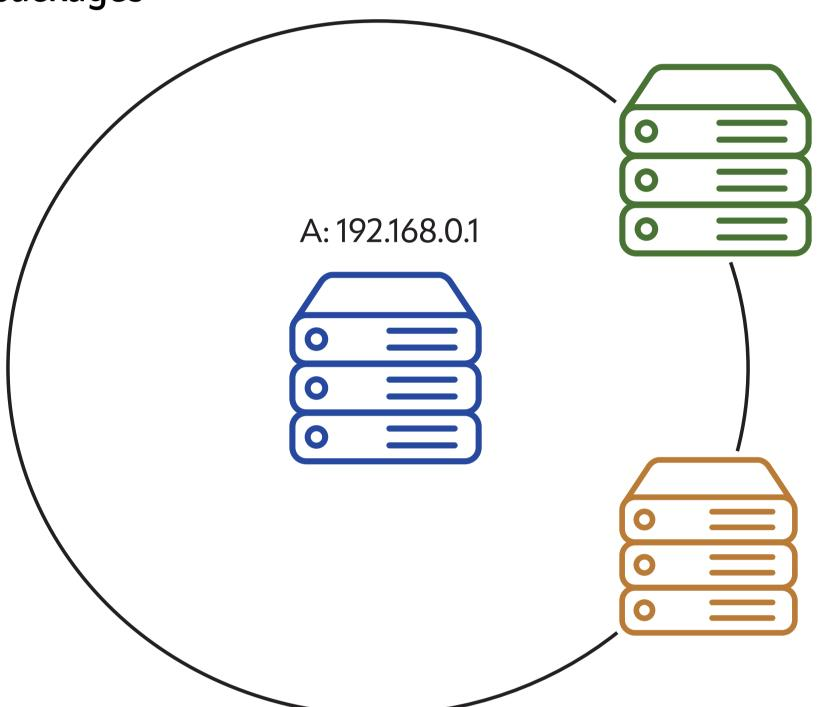
When a node stops receiving CARP packages for a while, another node decides to step in and become an active node. This situation is shown in Figure 3. The blue node, for some reason, stopped announcing the package, the green node noticed it, and now it has started to announce the CARP packages. When the blue node comes back, it will notice that the green node is now an active node and it will stay passive.
